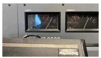
Test levels for external audio clips before airing, and adjust channel 'trim' knobs at the tops of the channels as necessary. This becomes especially important for phone calls, Zooms etc, as shown;
